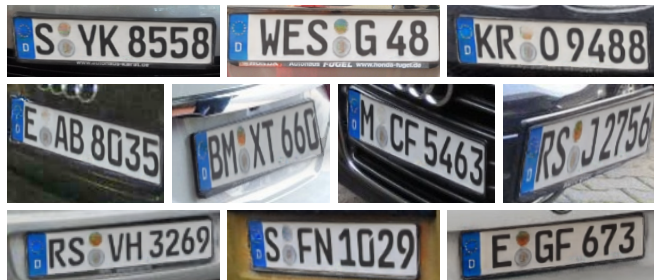
Fig. 1. Generated license plate samples. The proposed system is able to replace existing license plates with synthetic ones while, at the same time, preserving perspective, lighting condition, and sharpness of the original real-life image.
