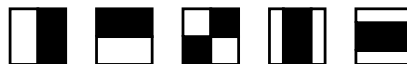
Figure 8: Haar features types used to generate one of the representations provided by the competition organizers.
